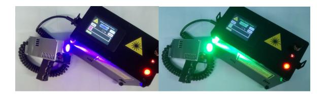
The **Revelation 445/520 nm Dual wavelength forensic** from Laser Innovations Ltd is a widely used a validated laser system for evidence recovery. The lightweight design (4 kg) provides 2 laser guns one Blue and one Green which are both easy to clean with 10% bleach solution. This laser provides 10 Watts Blue at 445nm and 8 Watts Green at 532nm.
